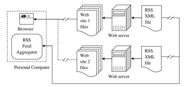
Fig 4.3: Communication between websites, RSS feed and PC
