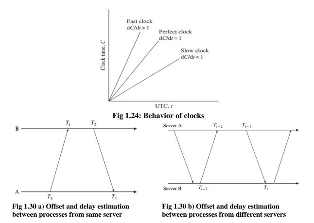
Let T1, T2, T3, T4 be the values of the four mostrecent timestamps. The clocks A and B are stable andrunning at the same speed. Let a = T1 - T3 and b = T2 - T4. If the networkdelay difference from A to B and from B to A, called **differential delay**, is small, the clock offset  $\theta$  and roundtrip delay $\delta$  of B relative to A at time T4 are approximately given by the following:
