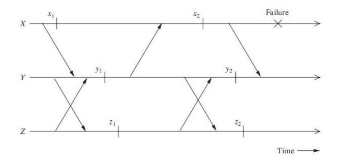
The above protocol, in the event of failure of process X, the above protocol will require processes X, Y, and Z to restart from checkpoints x2, y2, and z2, respectively.
