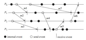
Fig 1.13: Asynchronous execution in message passing system
