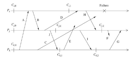
The computation comprises of three processes Pi, Pj , and Pk, connected through a communication network. The processes communicate solely by exchanging messages over fault-free, FIFO communication channels.
