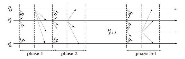
Fig. Message pattern for the phase-king algorithm.
