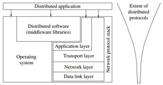
Fig 1.2: Interaction of layers of network
