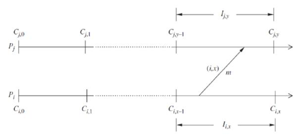
• When a failure occurs, the recovering process initiates rollback by broadcasting a *dependency request* message to collect all the dependency information maintained by each process.
