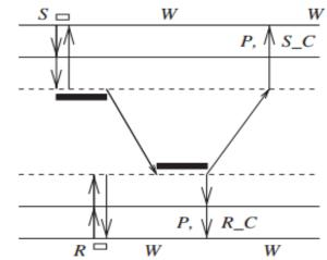
Fig 1.12 b) Non-blocking synchronous send and blocking receive
