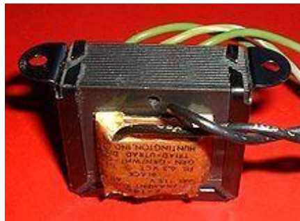
Figure 2.1 Laminated core transformer showing edge of laminations
