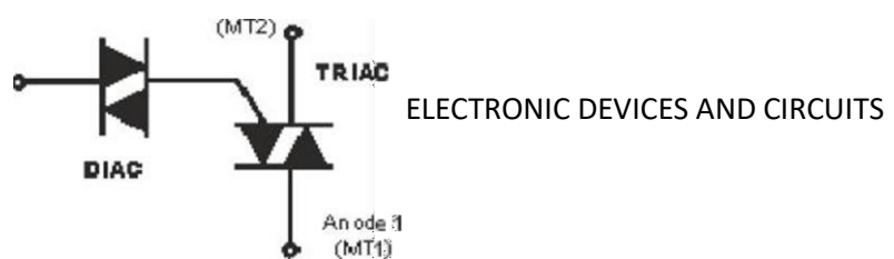
Figure 5.12 Typical DIAC / TRIAC circuit configuration
