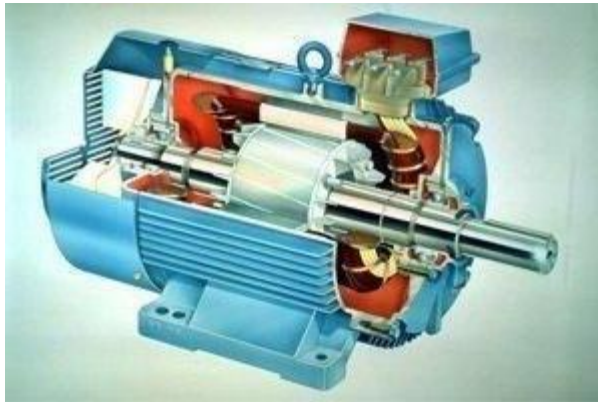
Fig. 8 Cut sectional view of the induction motor.
