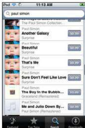
Figure 7-10. The scrollbar displays when the user starts scrolling through the content; the scrollbar is just a feedback mechanism to indicate scrolling is happening, how much content is loaded, and where the user is in the scroll operation
