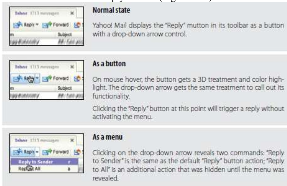
Figure 4-23. Yahoo! Mail’s “Reply” button looks like a drop-down when hovered over; clicking “Reply” replies to sender, and clicking the drop-down offers the default action as well as “Reply to All”
