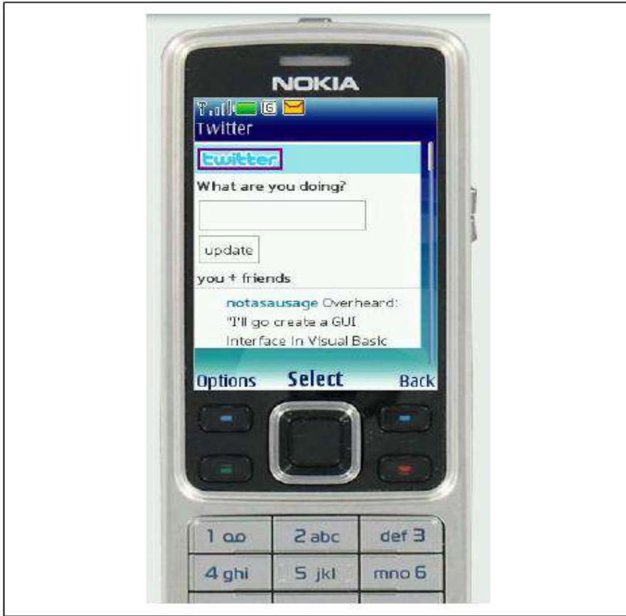
Figure 8-9. Example layout of a scroll-based application, where the user had to press the D-pad past each link to scroll the page
