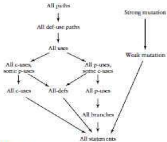
FIG. 5.5 A partial ordering for test adequacy criteria.
