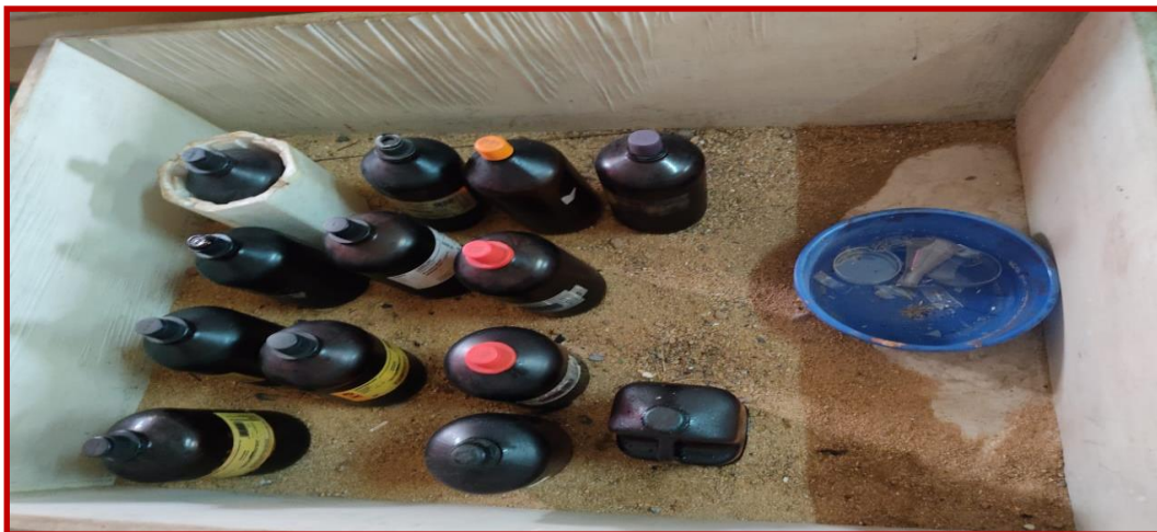
Fig. 4: Concentrated acids are stored in sand bed (Best practice)
