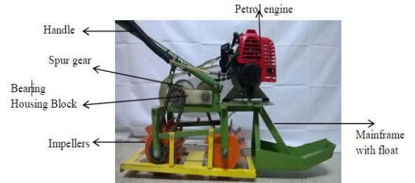
Figure 3.1: Details of Semi Automatic weeder
