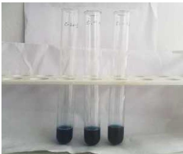
Fig.4.7(a) Test tubes showing blue color change for Bradford assay (1976).
