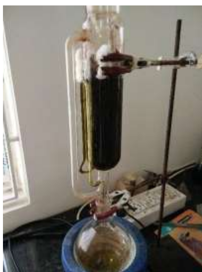
Fig:3.3 Extraction of Acalypha indica , Lawsonia inermis and Calotropis gigantea leaves using soxhlet extractor
